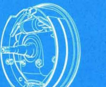
Air-Cooled Brakes for Safe, Positive Stopping! Durable, husky brakes are a vital part of sports car driving—and the Corvette's got the brakes to do the job! New slotted wheel discs permit air to cool the innermost areas of the big 11-inch hydraulic brakes, help maintain constant high-brake efficiency and add extra lining life, Brakes are self-energizing with faderesistant, bonded linings.
