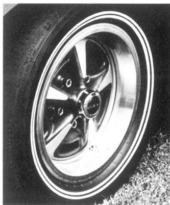
Rally II Wheels (Code 474—UPC N98). Available all models (except Catalina, Executive and Bonneville Station Wagons). 15-inch diameter for Catalina, Executive and Bonneville. 14-inch diameter on all other models. Stamped steel gives appearance of magnesium. Chrome-plated wheel nuts. (Conventional spare wheel provided with "Space-Saver Spare" Tire.) (F)
