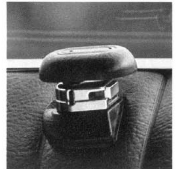
Rear-door Child Lock Guards (4-door models only). Children can't open or unlock rear doors when buttons are down and Lock Guards are in. Yet door can easily be "popped open" with a key. Any of regular car keys can be used. (Illustration 1—Unlocked position; 2—Regular Locked position; 3—Lock Guard position.) (D)
