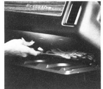
Glove Compartment Lamp (Code 664—UPC U27). Available Tempest and LeMans models only—included in Lamp Group (Code 322). Standard all other models, all series. Lights automatically when glove compartment door is opened. (F,D)
