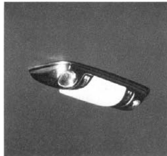
Dome Reading Lamp (Code 654—UPC C89). Consists of center lamp and two side lamps. Center unit operates as a conventional dome lamp from door jamb switches and headlamp switch knob. Side lamps operate from separate switches on lamp housing and shine over shoulders of front-seat occupants. Available all series. (F)
