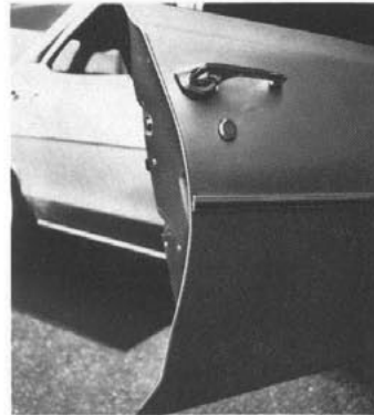
Door-edge Guards (Code 684—UPC B93). Bright, stainless steel strips help protect door edges from nicks and scratches. Available all models. (F,D)
