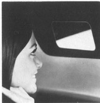
Visor Vanity Mirror (Code 441—UPC D34). Mounts on back of visor. Out of sight when not being used. Available for right and/or left visors, all models. (F,D)
