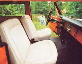
Bronco interior features: driver's bucket seat in parchment vinyl • floor insulation and mat (front and rear) with bright retainers • vent window handles • armrests • lockable glove compartment, and much more.
