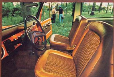
Bronco Ranger interior features, in addition to or in place of Sport Package, include: cut-pile front carpet • full rear carpeting • door trim panels • vinyl trim and insulation on rear quarter panels • interior trim in tan, blue or jade. Rear seat is required.
