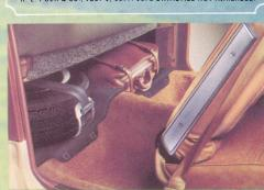
Concealed storage and spare tire compartment. Both sides of the split-back seat back fold down for easy access to in-cab storage area under the pickup box. The spare tire includes extractor for easy removal.
