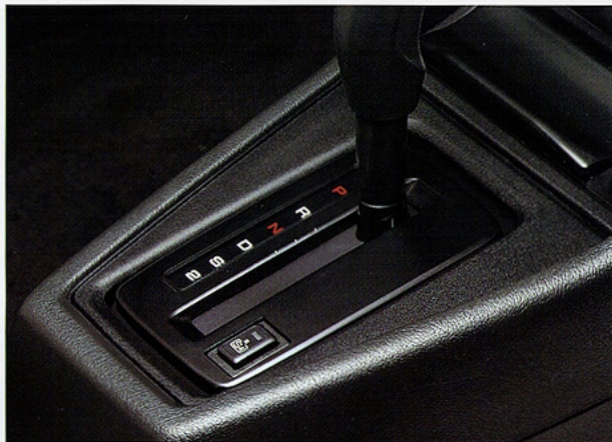
For less shifting between gears and improved engine braking, an electronically controlled 4-speed automatic transmission with sport shift is available.
