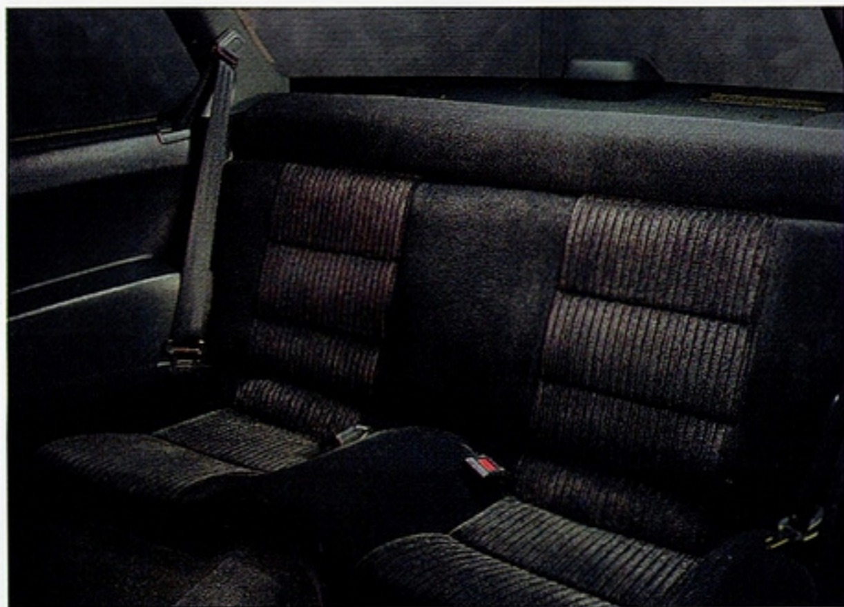
Three-point lap-shoulder belts keep passengers securely in their place. The rear seat also folds forward for direct access to the trunk.
