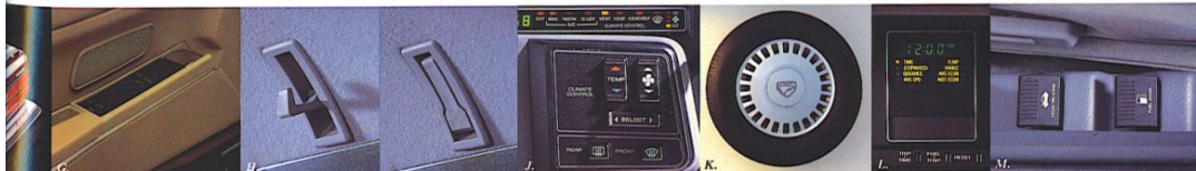
A. FM electronically tuned stereo cassette, separate seven-band graphic equalizer, and power antenna. B. Standard rear window defroster. C. Optional rear deck luggage rack. D. Recessed door lock controls (included with optional Power Lock Group). E. Seven-function trip computer (included with Electronic Information Package; standard ES, optional LX). F. Floor-mounted remote release for hood and fuel door (fuel door release included with optional Power Lock Group).
