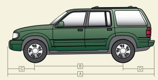
A Overall length measures from the rear bumper to the front bumper. B Wheelbase measures the distance between the centers of the front and rear wheels (or axle). C Front overhang measures the distance from center of the front wheel (or axles) to front bumper. D Rear overhang measures the distance from center of the rear wheel (or axle) to rear bumper.
