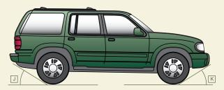
J Angle of departure measures the angle between the ground from the trailing edge of the rear bumper (or lowest rear component) to a tangent with the rear tire. K Angle of approach measures the angle between the ground from the leading edge of the front bumper (or lowest front component) to a tangent with the front tire.
