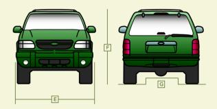
E Overall width measures the widest point at the sides of the vehicle excluding mirrors. F Height measures from the ground to the highest point on the roof of the empty vehicle. G Ground clearance measures between the ground and the lowest point of the vehicle.
