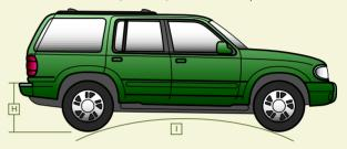
H Load floor height measures the distance from ground to cargo floor. I Ramp breakover angle measures the maximum angle of a rise that the vehicle can clear between its front and rear wheels.
