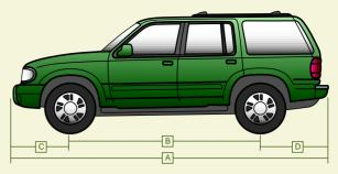
A Overall length measures from the rear bumper to the front bumper. B Wheelbase measures the distance between the centers of the front and rear wheels (or axle). C Front overhang measures the distance from center of the front wheel (or axles) to front bumper. D Rear overhang measures the distance from center of the rear wheel (or axle) to rear bumper.
