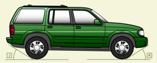
Angle of departure measures the angle between the ground from the trailing edge of the rear bumper (or lowest rear component) to a tangent with the rear tire. K Angle of approach measures the angle between the ground from the leading edge of the front bumper (or lowest front component) to a tangent with the front tire.
