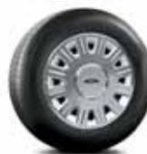
16" Steel Wheel with Cross-Spoke Locking Wheel Cover
