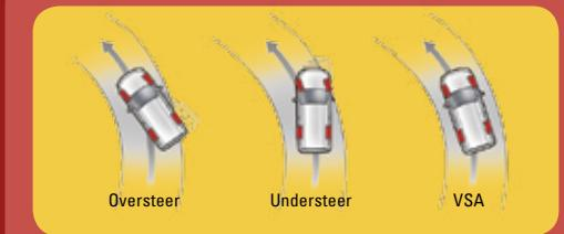
Vehicle Stability Assist (VSA) can help detect oversteer or understeer, to help restore the driver's intended path.
