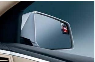
Blind spot mirrors, integrated into the outside mirrors, are standard on LT and LTZ. Designed to enhance visibility along the sides of the vehicle, this forward-thinking feature is just one more way Traverse helps surround you in safety.
