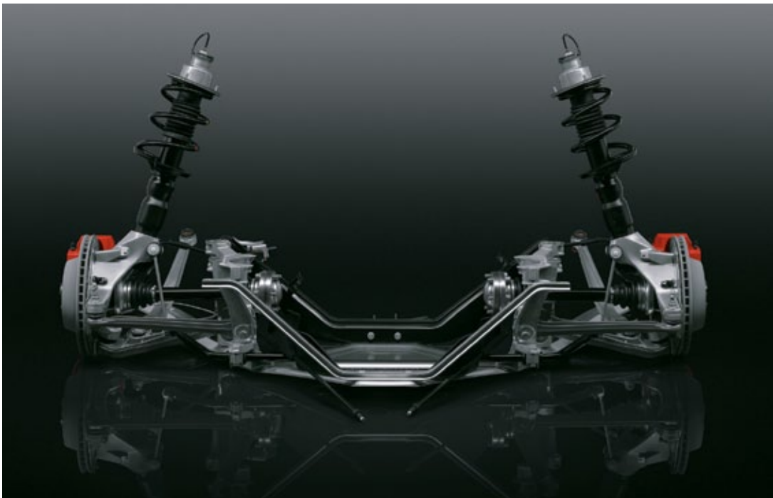
Lightweight spring-strut rear axle on the Cayman S
