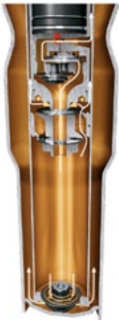
Compression in Normal mode—working piston and bypass, sporty-comfortable tuning
