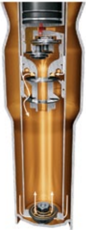
Rebound in Sport mode—working piston only, sporty-hard tuning
