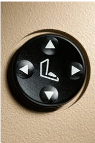
Lumbar support for front seats adds four-way adjustable comfort for the lower back. Lumbar support can be adjusted up/down and in/out.
