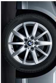
Star Spoke (Style 286) light alloy wheels with run-flat 2 performance tires . 3 In front: 17 x 8.0 wheels with 225/45 tires; in back: 17 x 8.5 wheels with 225/40 tires.
