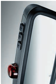
BMW Universal garage-door opener takes the place of up to three remote-control devices. It can activate remote functions outside the vehicle, such as garage-door openers or home-lighting systems.
