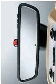
The automatic-dimming inside rear-view mirror darkens in response to the bright headlights of vehicles behind you. The easy-to-read digital compass , integrated into the mirror, is a convenient way to constantly keep your bearings while driving.
