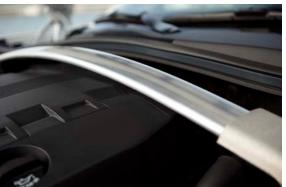
How you feel behind the wheel is everything in a Camaro, and driving a convertible is no different. That's why the Convertible features an aluminum tower-to-tower brace combined with a pair of underbody V-braces for added reinforcement.
