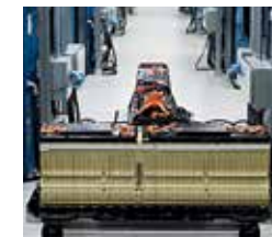
Uncovered look at the 288-cell lithium-ion battery pack.
