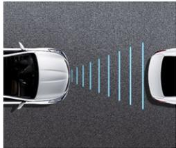
**FORWARD THINKING** Azera Limited comes standard with a new Forward Collision Warning System that senses the potential for a collision with a vehicle in front of you and sounds an alarm. The warning signals the driver to apply brakes to help prevent a collision or mitigate its impact. A new Lane Departure Warning alerts the driver when the car drifts from its driving lane.
