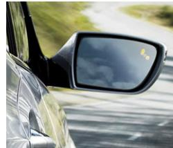
**BLIND SPOT DETECTION** New for 2015, this technology warns the driver of an approaching vehicle using indicators on the side mirrors or, if needed, an audible warning. Lane Change Assist factors the speed of adjacent vehicles into the warning calculus when you're switching lanes.
