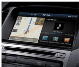
**ADVANCED NAVIGATION** Azera's high-resolution 8" touchscreen includes a new split-screen feature that displays navigation and audio functions simultaneously. The advanced navigation system includes voice-command control and junction view lane guidance. Need help backing into parking spaces? The screen also serves as a monitor for the integrated rearview camera.
