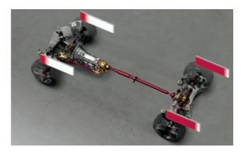
In normal driving conditions, virtually all torque is distributed to the rear wheels providing signature Jaguar rear wheel drive performance.
