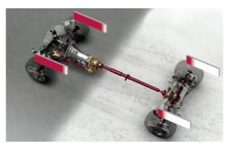
Where road conditions are changing, up to 100% of torque can be distributed to the front wheels as required to ensure optimum traction.
