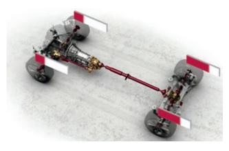
At the touch of a button Winter Mode can be selected to automatically distribute 30% of the torque to the front wheels and 70% of the torque to the rear wheels maximising control in difficult conditions.
