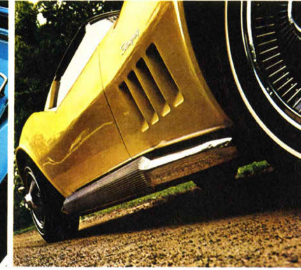
Side-mounted exhaust system.
