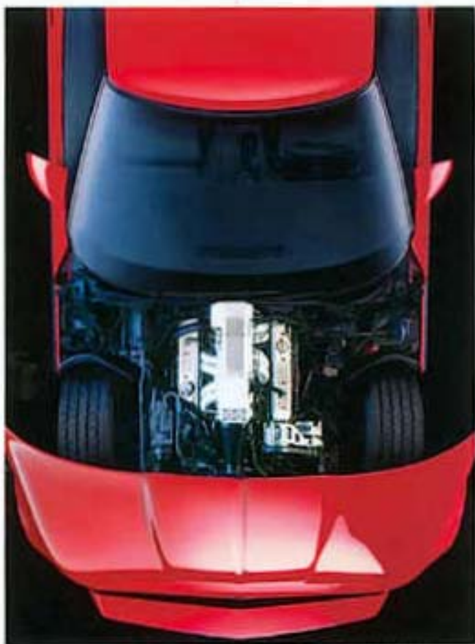
Corvette's 5.7 Liter V8 with Tuned Port Fuel Injection delivers 245 HP at 4300 RPM.*
