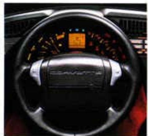
The new-for-1990 Supplemental Inflation Restraint system (air bag) is located in the hub of the steering wheel. The S.I.R. is designed to provide added protection to the driver in the event that your Corvette is involved in a moderate to severe frontal impact. For maximum protection in frontal and all other collisions, both driver and passenger should be properly restrained with safety belts.
