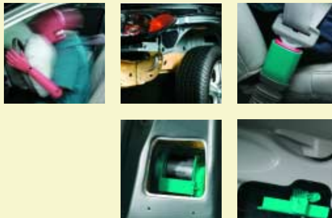
Our standard Personal Safety System includes (clockwise from upper left) dual-stage front airbags, crash severity sensor, safety belt usage sensors, driver seat position sensor, safety belt energy management retractors and safety belt pretensioners.
