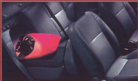
60/40 rear seat with flip-up rear cushion, standard on all Focus models. Shown with optional leather trim.
