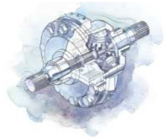
Baja models feature a standard limited-slip rear differential that further enhances traction. If one rear wheel starts to lose traction, power is automatically diverted to the other rear wheel—all without the need for driver intervention.
