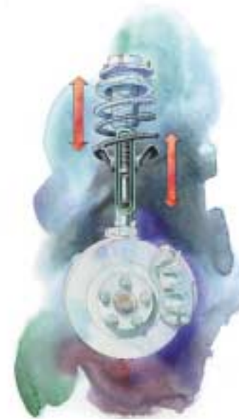
As the body of a vehicle leans in a turn, the suspension of the inside wheels extends. All Baja models feature a rebound spring inside the front strut that is designed to use the mass of the wheels, tires and brakes to resist this extension, reducing body roll in turns. The rebound spring also works to reduce the lift of the nose of the vehicle during acceleration.
