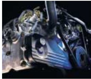
Baja is powered by a 2.5-liter, 16-valve horizontally opposed boxer engine producing 165 horsepower and 166 lb.-ft. of low-end torque.
