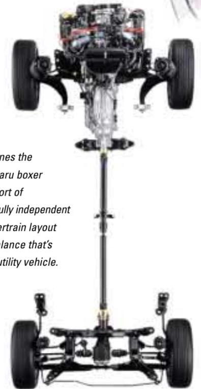
Symmetrical All-Wheel Drive combines the lower center of gravity of the Subaru boxer engine with the control and comfort of low-friction, long travel, 4-wheel fully independent suspension. A symmetrical powertrain layout gives Baja models a sense of balance that's more like a sport sedan than a utility vehicle.
