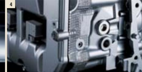
**4** Aluminum-alloy block and cylinder heads help to reduce weight, improving overall vehicle balance without sacrificing strength or durability.
