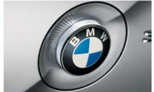
■ **Side indicator lights** with white lenses. When flashing, the light radiates outward from behind BMW's signature roundel.
