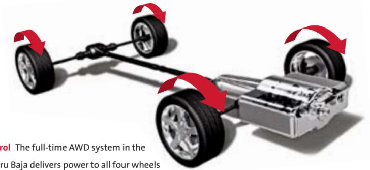
**Control** The full-time AWD system in the Subaru Baja delivers power to all four wheels continuously, resulting in greater traction for more predictable handling. When slippage is detected, the system instantly transfers power from the wheels with the least amount of grip to the ones with the most. Enhanced adhesion. Maximum safety. More peace of mind.
