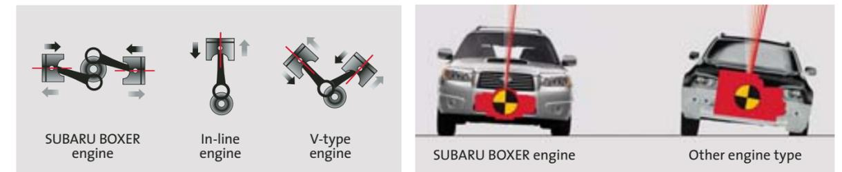
**Less vibration** The 180-degree boxer engine layout allows the pistons to move in exact horizontal opposition, effectively negating the vibrations of the opposing pistons. The result is smooth, seamless power delivery throughout the rev range.
