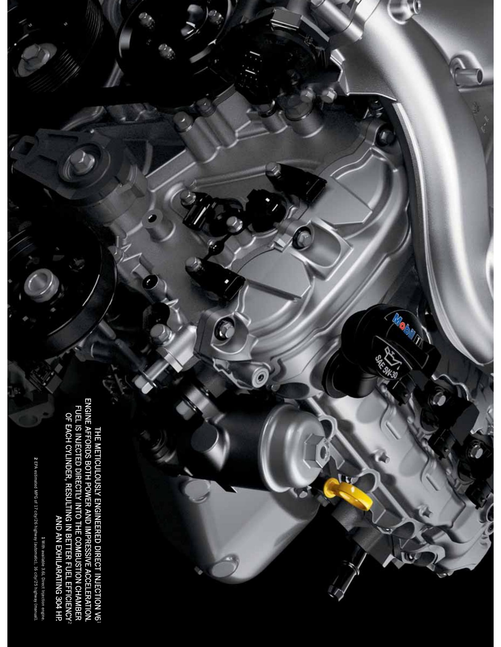
THE METICULOUSLY ENGINEERED DIRECT INJECTION V6<sup>1</sup> ENGINE AFFORDS BOTH POWER AND IMPRESSIVE ACCELERATION. FUEL IS INJECTED DIRECTLY INTO THE COMBUSTION CHAMBER OF EACH CYLINDER, RESULTING IN BETTER FUEL EFFICIENCY<sup>2</sup> AND AN EXHILARATING 304 HP.
