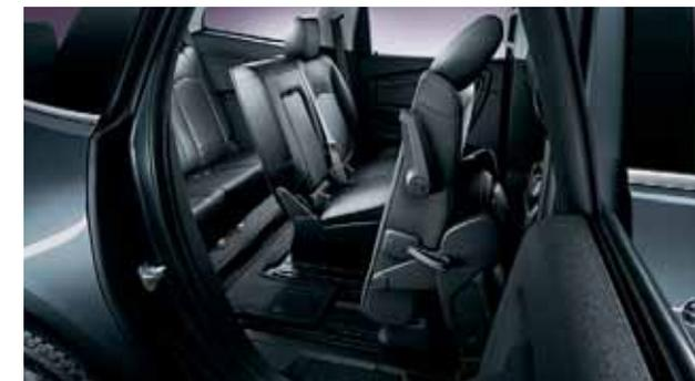
A one-hand movement sends the Smart Slide second-row seat into motion, quickly sliding it out of the way and allowing passengers of all ages and sizes to easily enter or exit the third row.
