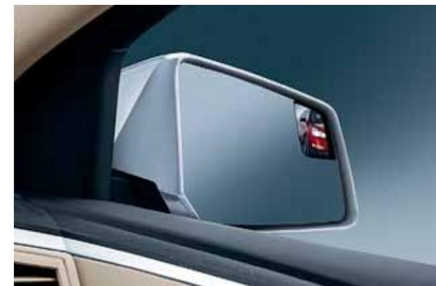
Blind spot mirrors, integrated into the outside mirrors, are standard on LT and LTZ. Designed to enhance visibility along the sides of the vehicle, this forward-thinking feature is just one more way Traverse helps surround you in safety.
