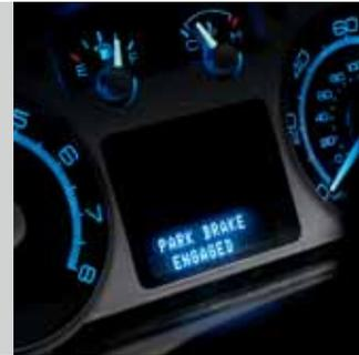
**Consideration.** A standard message center, located between the tachometer and speedometer, displays trip computer readings and other vital information. Check your messages frequently.
