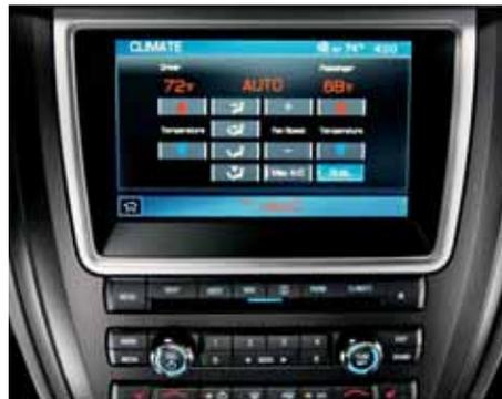
**Activation.** On models equipped with Milan's available voice-activated touch-screen Navigation System, the Dual-zone Electronic Automatic Temperature Control can be operated 2 ways: by voice (say "Temperature Up" or "Temperature Down"); or by touching the up or down arrows on the Navigation System's Climate screen.
