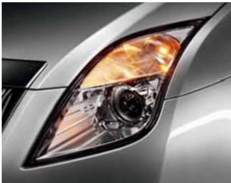
**Illumination.** An automatic headlamps feature on Milan Premier and Milan Hybrid turns the headlamps on and off automatically based on ambient light conditions.
