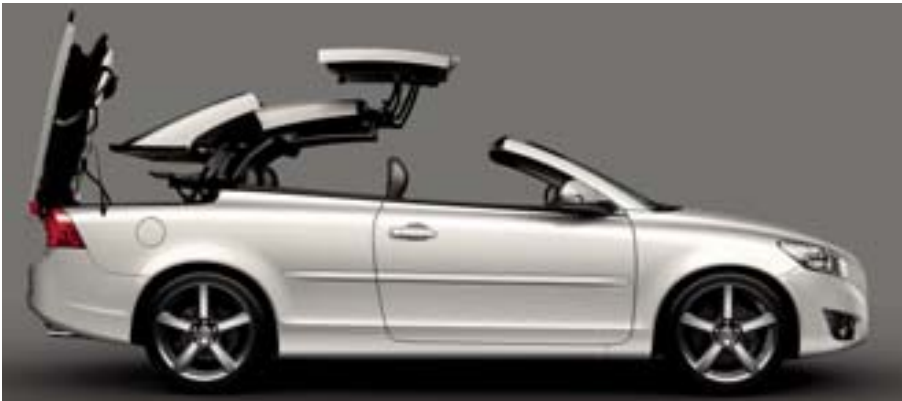
Three-split retractable hardtop
