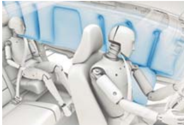
Inflatable Curtain (IC)
